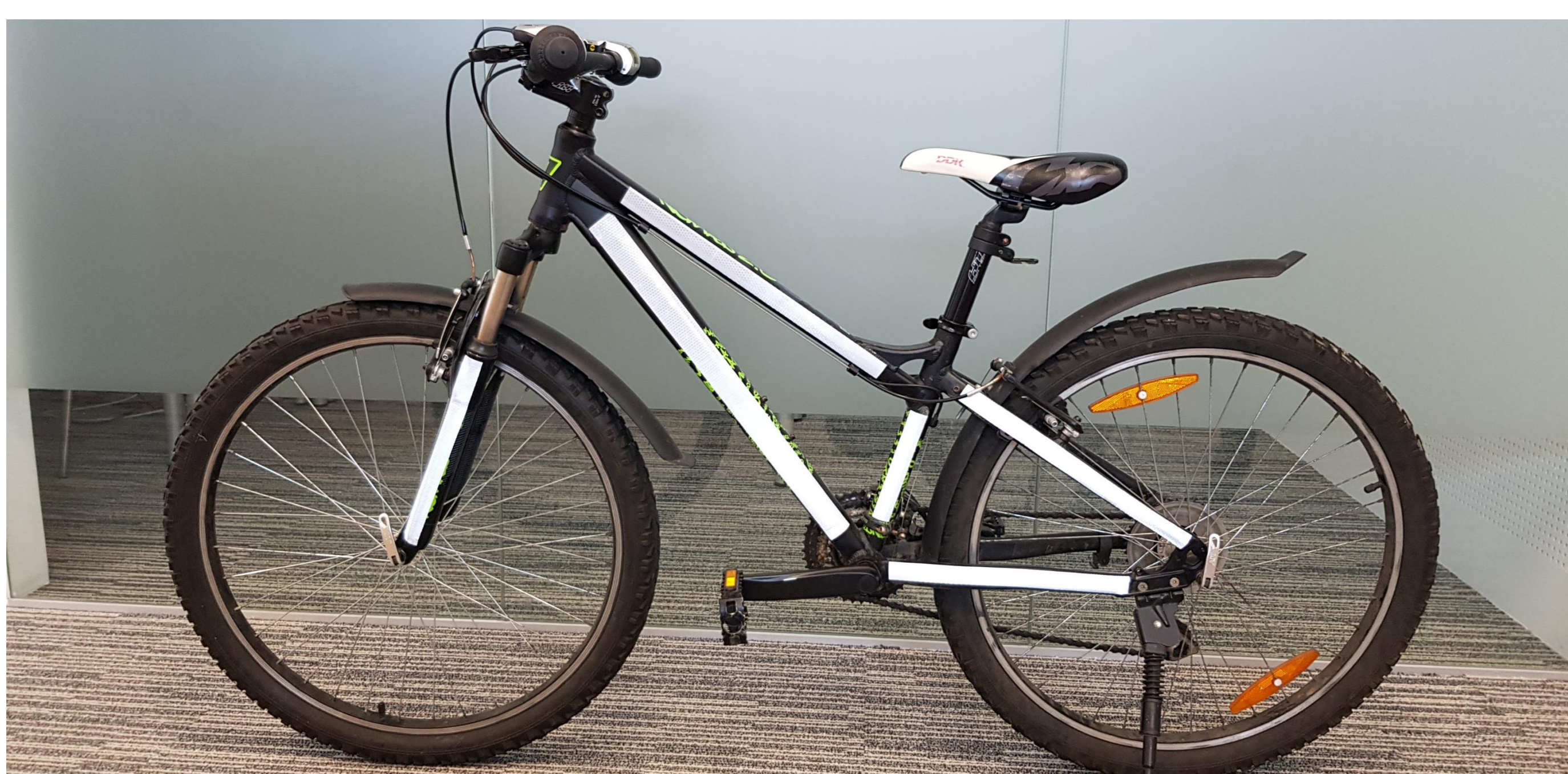
Fig 2. Bicycle equipped with proposed retro-reflective pattern
