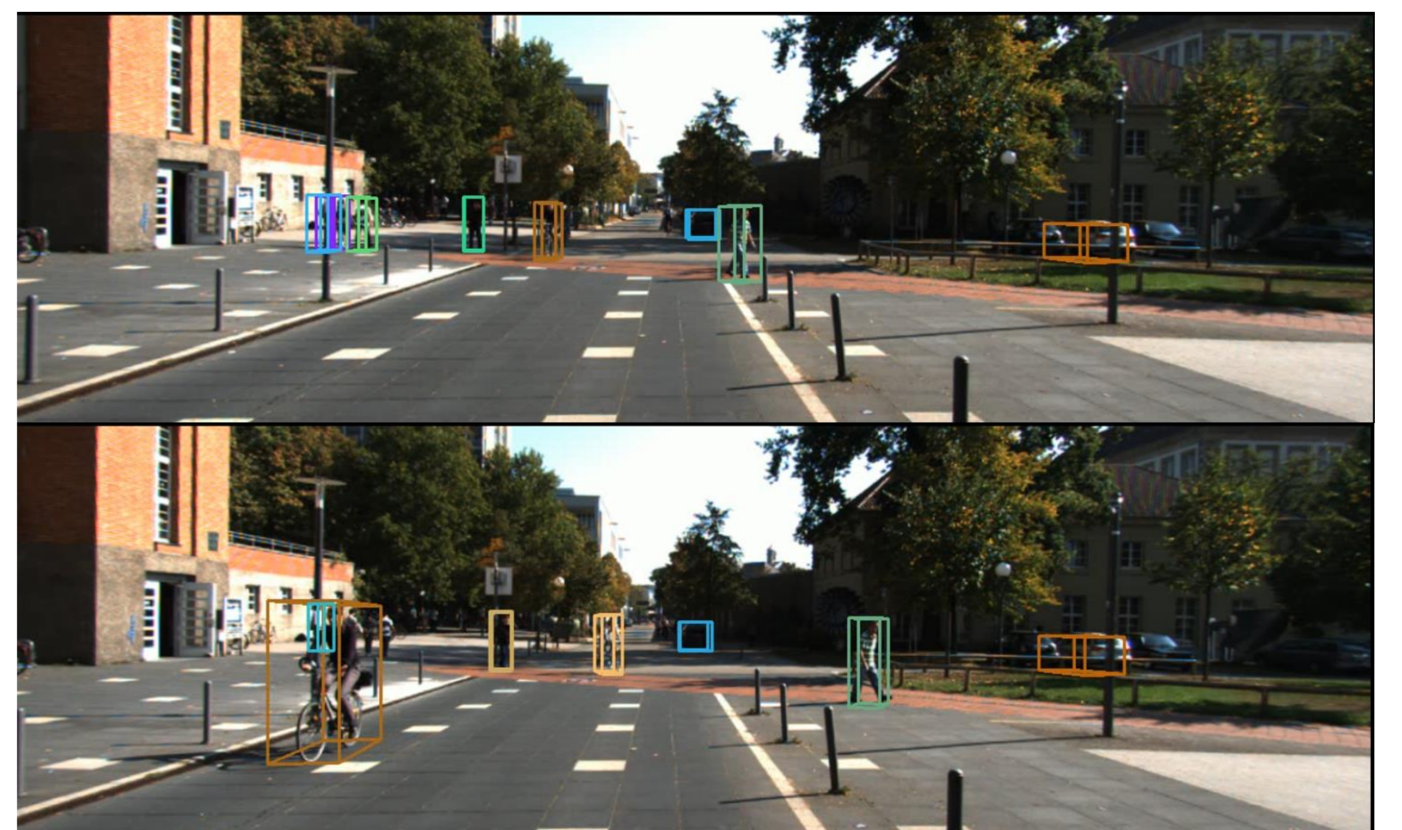
Fig 3. Monocular pose estimation and tracking results using our baseline
