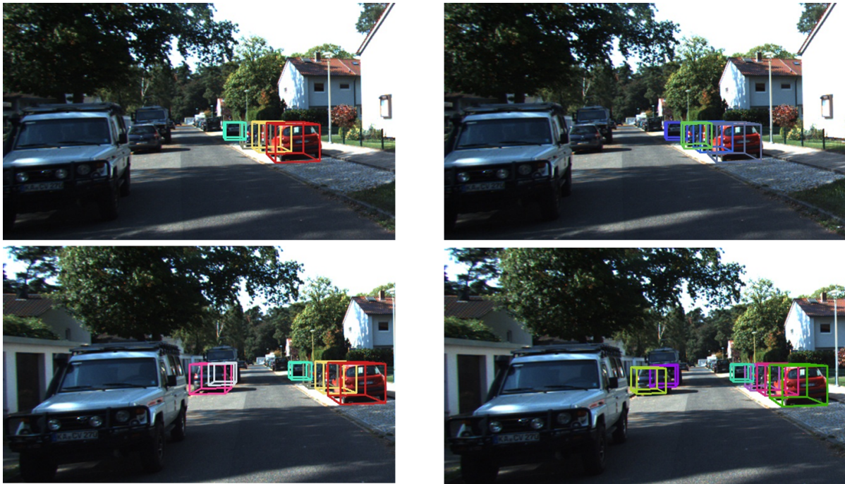
Figure 4: Comparison between proposed reID approach (left) and simple Kalman Filter (right) on the KITTI validation set.
